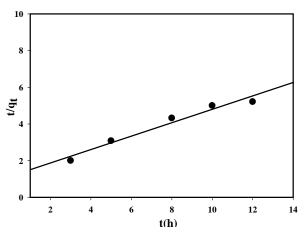
Figure 7. Pseudo- second order kinetics plot for the adsorption of Remazol Red on saw dust at 25°C.
