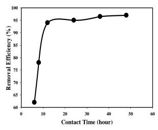
Figure 2. Effect of contact time on the removal of RR. Particle size: 140μm; Adsorbent amount: 1.0 g; Initial conc.: 50 mg/l; Initial volume: 50 ml; pH: 7.0; Temp.: 25<sup>0</sup>C.
