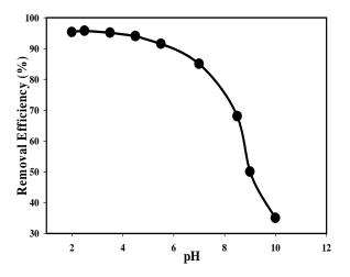
Figure 3. Effect of pH on the adsorption capacity of saw dust for Remazol red at 25<sup>o</sup>C.
