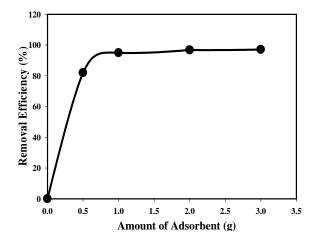
Figure 3. Effect of adsorbent amount on the removal of RR. Particle size: 140 μm; Initial concentration: 50 mg/l; Initial volume: 50 ml; pH: 7.0; Contact time: 12 hours; Temp.: 25<sup>0</sup>C.
