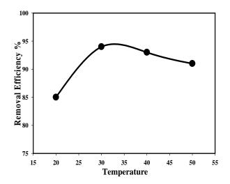
Figure 4. Effect of temperature on the removal of RR. Particle size: 140μm; Adsorbent amount: 1.0 g; Initial conc.: 50 mg/L; Initial volume: 50 ml; pH: 7; Contact time: 12 hours.
