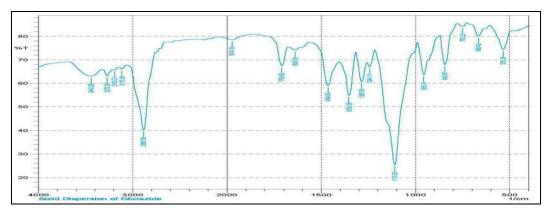
Figure 4. FT-IR spectrum of solid dispersion of gliclazide (SD1/5).
