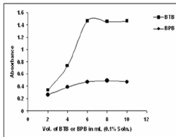
Figure 3. Effect of dye concentration on ion pair complex.
