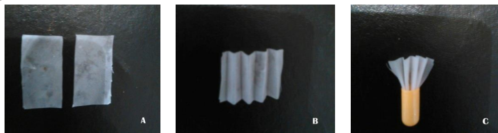
Figure 1. (A) Film of enalapril maleate, (B) Zigzag folding pattern, (C) Film inserted into '00' size capsule shell.
